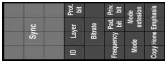
Figure 2: MP3 Header composition
