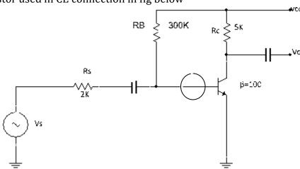
Has the following set of h-parameters : $h_{ie}$ =1K, $h_{fe}$ =100, $h_{re}$ =5x10<sup>-4</sup> and  $h_{oe}$ =2x10<sup>-5</sup>s with R<sub>s</sub>=2K and R<sub>c</sub>=5K,determine
