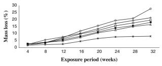
Fig. 2 Percentage mass losses of wood specimens in the fungal soil-bed
