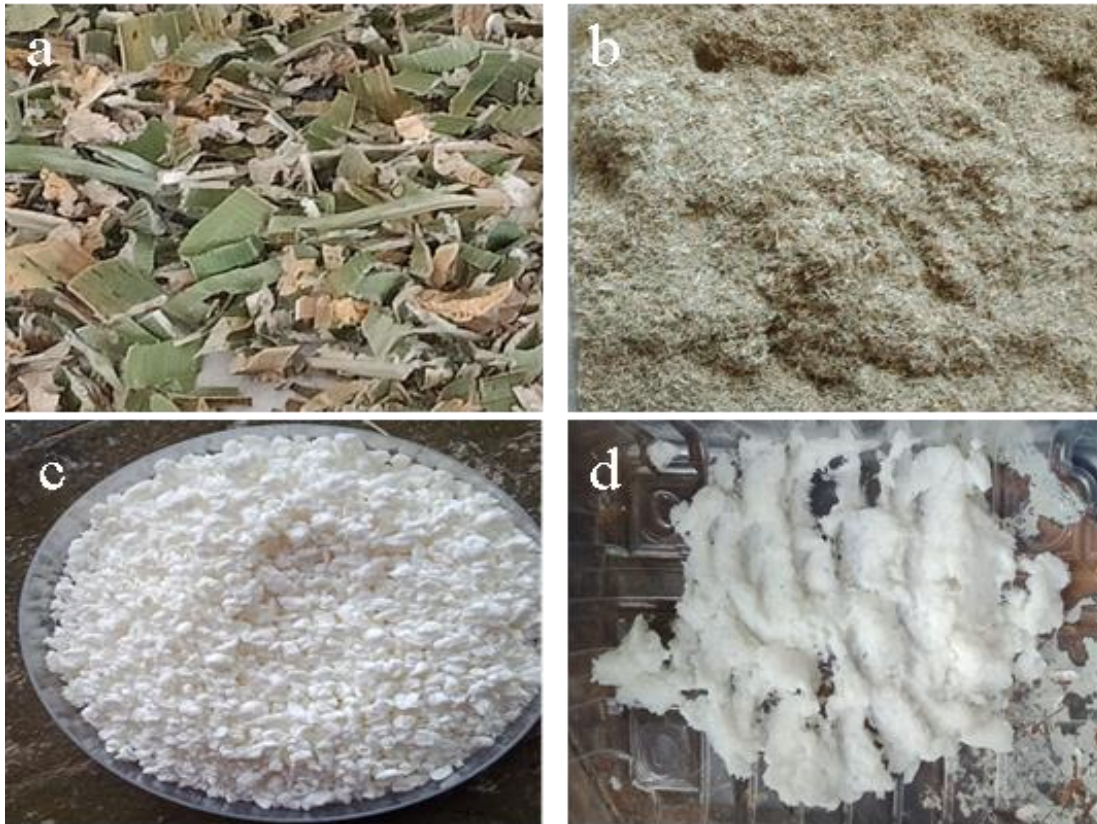
Figure 4.1: Physical appearance of (a) Chopped Typha angustifolia , (b) Crushed Typha angustifolia , (c) Isolated cellulose and (d) Cellulose nanocrystals
