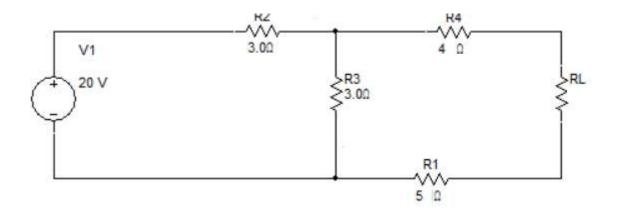
b) Determine equivalent resistance in the arrangement shown below (4 marks)
