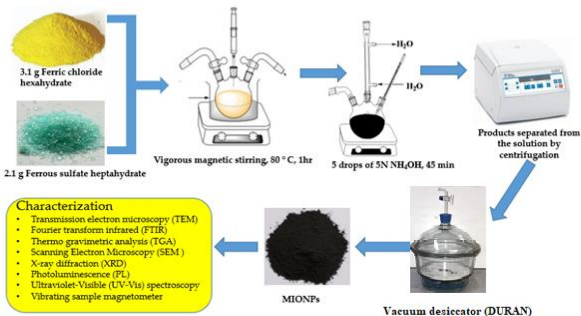
Fig.1. Flow diagram for the synthesis of MIONPs
