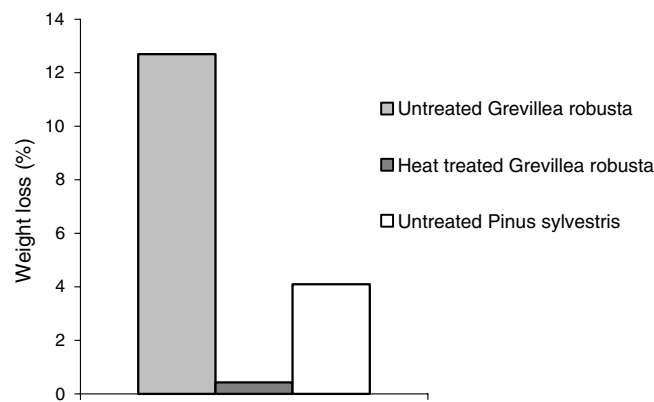
Fig. 7. Weight losses of Grevillea robusta heat treated for 7 h at 250 °C and controls tested against termites in laboratory conditions for 28 days.
