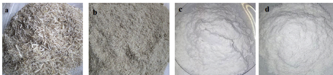
Fig. 1. Physical appearance of collected sugarcane bagasse (a), crushed sugarcane bagasse (b), extracted cellulose (c) and nanocrystals (d).
