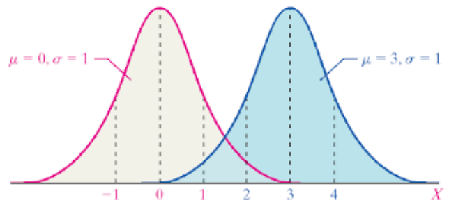
Figure 5. Shift of the normal curve towards the outlier changing the mean but keeping the standard deviation constant.
