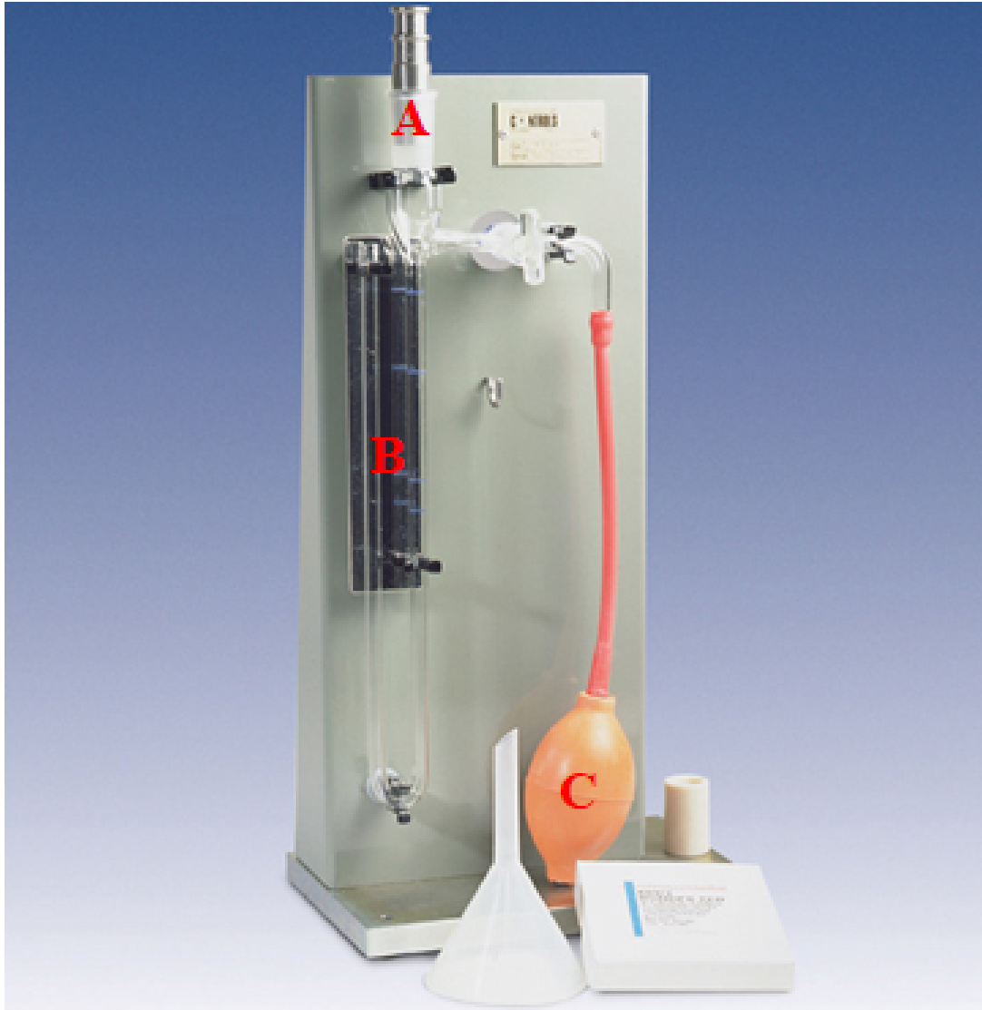
Figure 4.8: A photograph of the Blaine Analyzer (CM/L 0278348) that was used in this work. (Courtesy of East African Portland Cement Ltd., Athi River, Kenya). The parts labelled A - shows the sample compartment, B - the U-manometer, C - rubber bulb.
