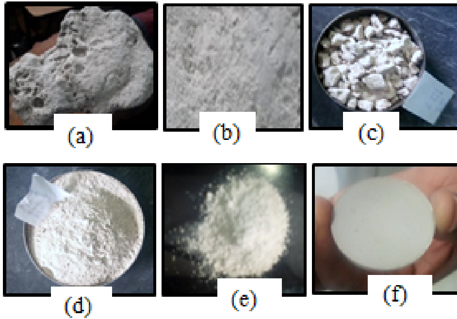
Figure 4.2: Schematic representation of the sample preparation steps: (a) As-collected sample, (b) Cleaned rock, (c) Crushed to sizes of 10 – 20 mm, (d) Pulverizing to the size of < 1000 \mu\text{m} , (e) Sifted dust of micron-size particles, (f) Pelletizing to the size of 5 mm-thick and 22 mm-wide discs
