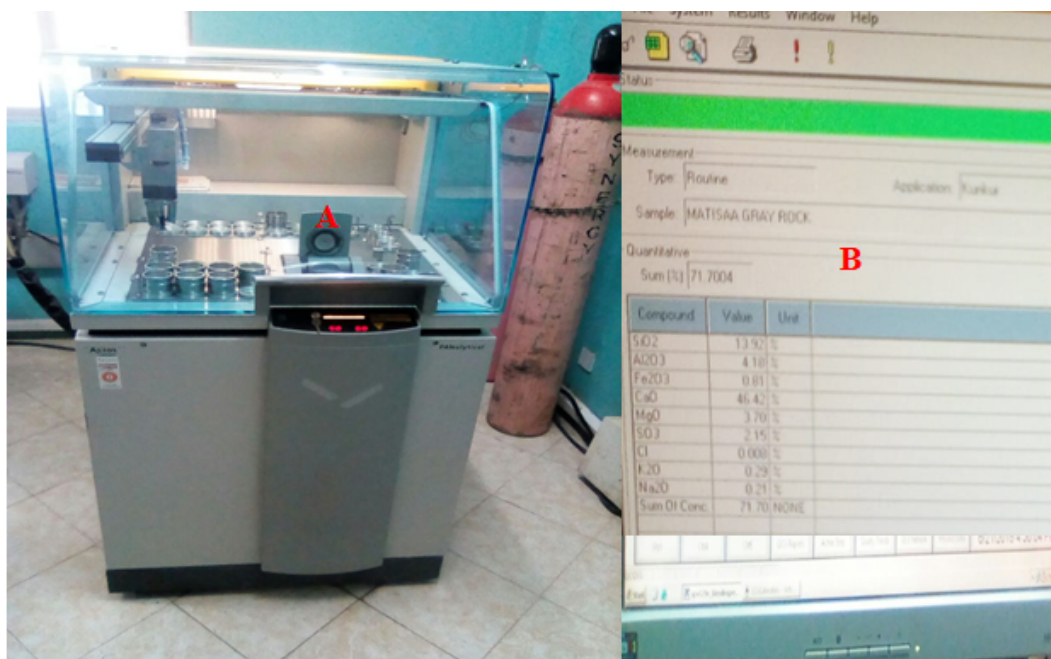
Figure 4.4: A photograph of the WDXRF instrument (PANalytical AXIOS) that was used in this work. (Courtesy of East African Portland Cement Ltd., Athi River, Kenya). The parts labelled A - shows the sample chamber, and B - the display.
